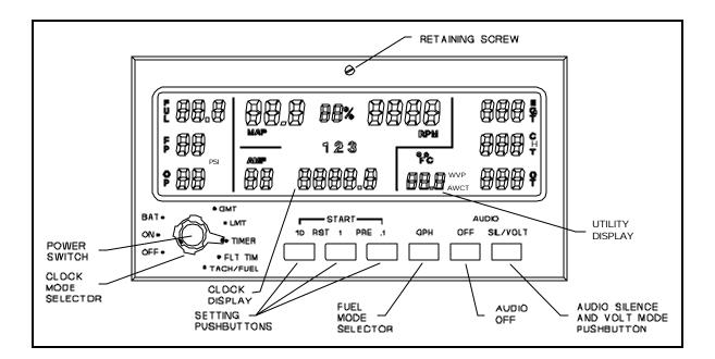
The gray pushbuttons are momentary switches that have to be held in to accomplish their function. The two yellow pushbuttons are push-push switches that alternately lock in when pushed and then release when pushed again. When either yellow pushbutton is 'in' it activates the function that is printed directly above it. The utility portion of the display shows optional functions such as carburetor temperature, outside air temperature and voltage.
